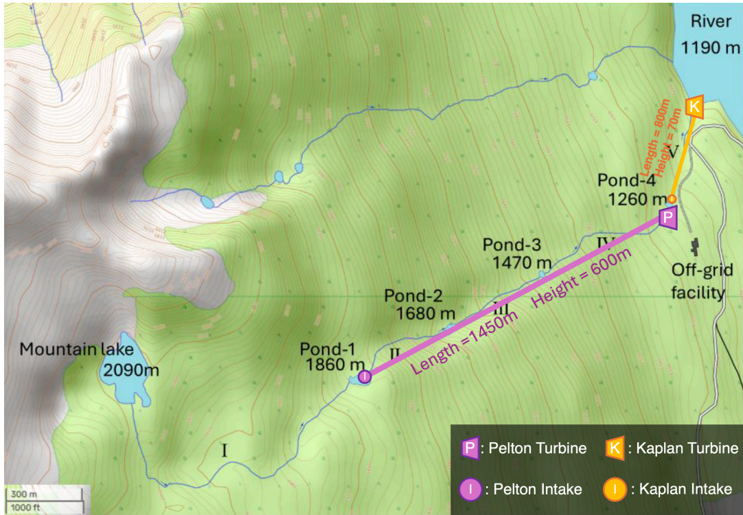
Figure 3: 2P5K Double Turbine Hydroelectric Design Concept Overlay
